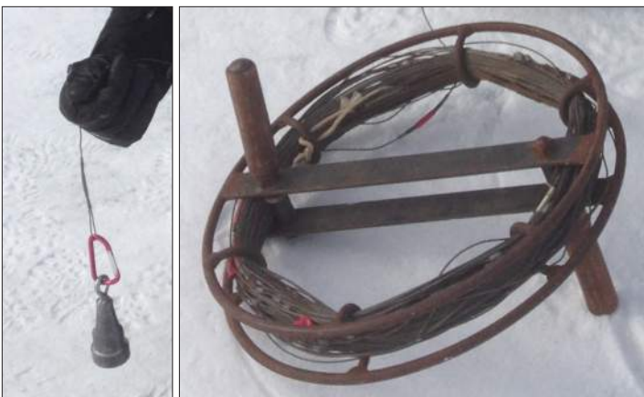
Figure 1. Weighted depth sounding line. (Left: weight; right: line on reel.)
